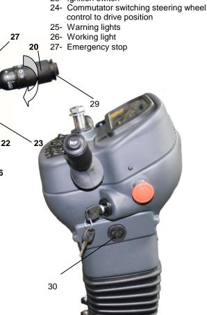
21- Rotary lamp 22- Working light 23- Ignition switch
